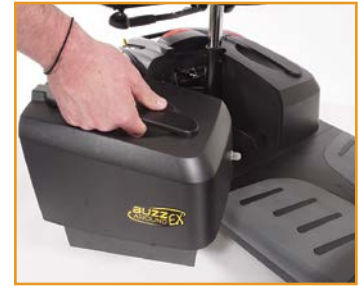
Step 2: Pull out the battery pack!
